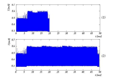
Figure 8: (1) Encryption of message M using exponent  $e=(07)_{16}.$  (2) Encryption of message M using exponent  $\hat{e}=({\rm FF})_{16}.$
