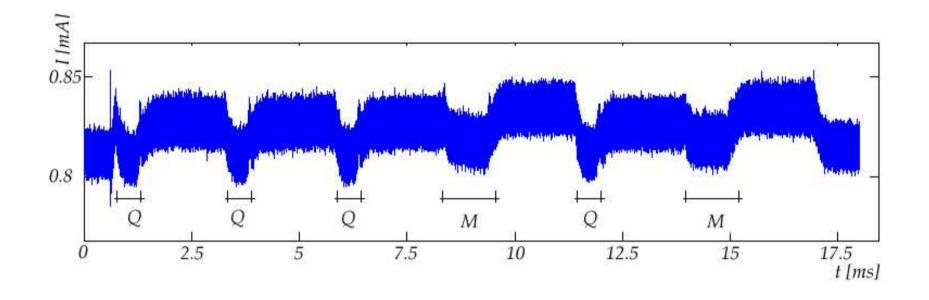
FIGURE 6: MEANTRACE FOR 100 TRACES. Q LABELS AN SECTION FOR A SQUARING DOWN, M LABELS A SECTION FOR A MULTIPLICATION.
